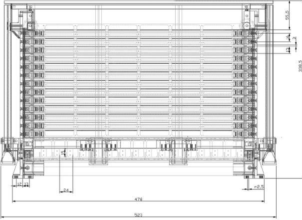
**Fig. 1.** Lateral cross-section of the AGILE baseline instrument. The anticoincidence system of plastic scintillator panels surrounds the detector made of 10 W-Si planes ( $0.7 X_0$ ) plus 2 more Si-only planes and a CsI mini-calorimeter ( $1.5 X_0$ ). The baseline payload size is  $\sim 53 \times 53 \times 35 \text{ cm}^3$ , and  $\sim 53 \times 53 \times 44 \text{ cm}^3$  for Super-AGILE
