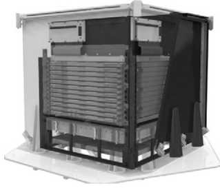
Fig. 1. Schematic view of AGILE Scientific Payload. SA is placed on the top of the payload, 12 trays of ST are placed in the middle and the MCAL is placed on the bottom of the payload, with detection planes facing ST and electric broad facing satellite shell.
