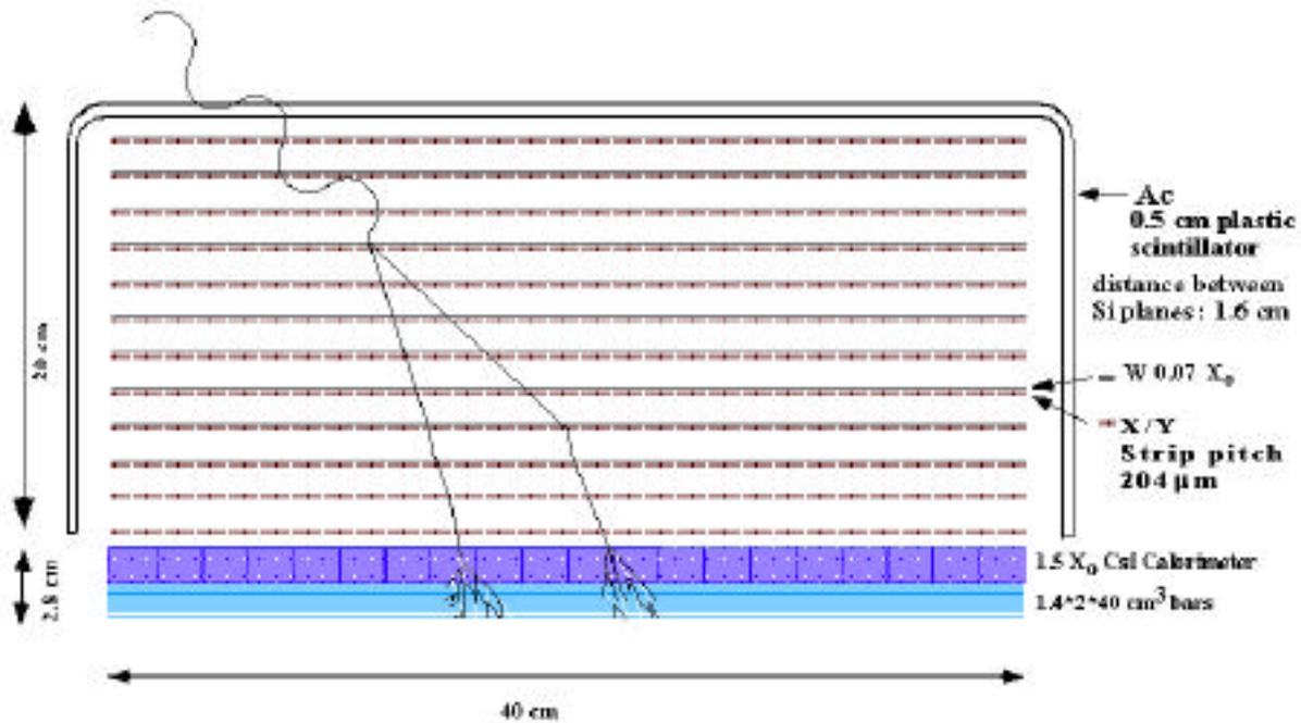
Figure 1: Schematic of the AGILE baseline instrument.
