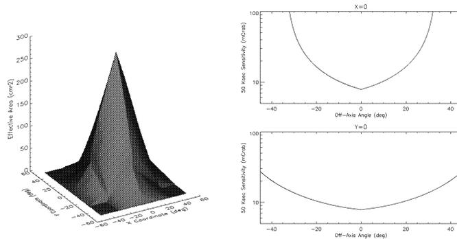
**FIGURE 3.** *Left Panel:* Effective area of 4 Super-AGILE detector units over the FOV. *Right Panel:* 50  $\sigma$  sensitivity of one Super-AGILE detector over the FOV for a 50 ksec observation
