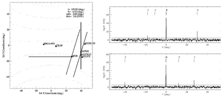
**FIGURE 4.** *Left Panel:* Simulated observation of a field near the Crab source. See the main text for the explanations. *Right Panel:* Super-AGILE sky images of a sample field with 5 sources. Each image, which is a combination of two detectors was attitude corrected for spacecraft pointing errors.
