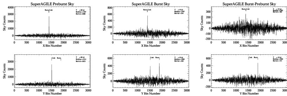
FIGURE 2. Illustration of possible on-board burst localizations by the Data Handling system. *Left:* X and Y sky images, integrated during the last 60 seconds before the burst trigger. The Crab pulsar is visible near the center of the field of view. *Center:* X and Y sky images obtained during 10 seconds of the burst. *Right:* The Data Handling system will be capable of normalizing the pre-burst data and subtracting it from the burst images, with consecutive determination of the burst position.
