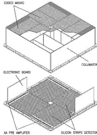
FIGURE 1. Schematic view of the Super-AGILE structure.
