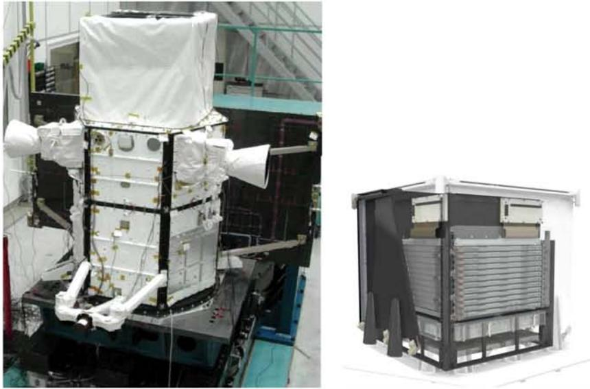
**FIGURE 1.** *Left panel:* The integrated AGILE satellite in its final configuration. The total satellite mass is equal to 350 kg. *Right panel:* the AGILE scientific instrument showing the hard X-ray imager, the gamma-ray Tracker, and Calorimeter. The Anticoincidence system is partially displayed, and no lateral electronic boards and harness are shown for simplicity. The AGILE instrument "core" is approximately a cube of about 60 cm size and of weight equal to 100 kg.
