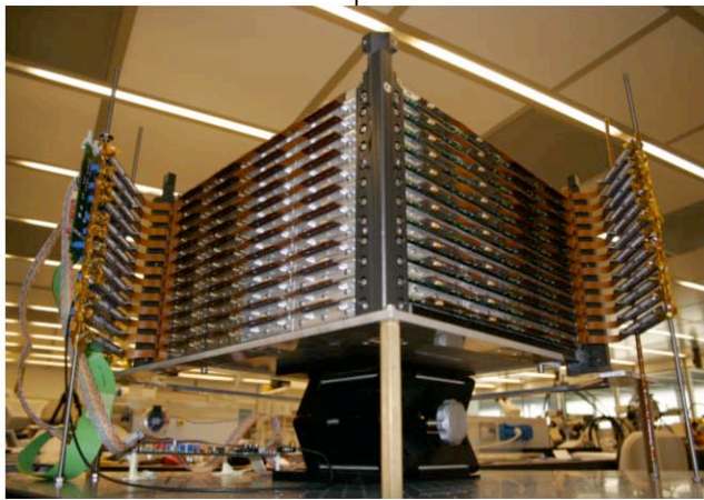
Figure 2. Left panel: the assembled AGILE Silicon Tracker developed by the INFN laboratories of Trieste before being integrated with the rest of the instrument (June 2005). Right panel: an example of an "environmental" gamma-ray event produced by cosmic-rays and detected by the Tracker with its characteristic pattern of released energy in clusters of hit readout Silicon microstrips (August 2005).
