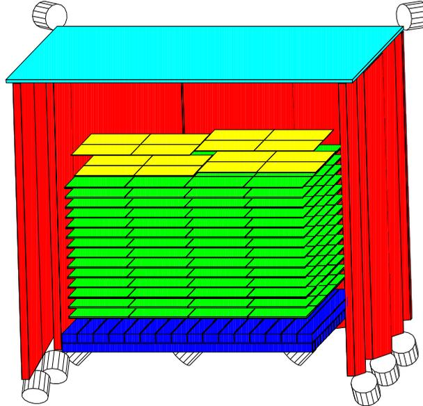
**FIGURE 1.** A simplified view of the AGILE instrument model. The Super-AGILE coded mask structure, the mechanical structure and the lateral electronics boards are not shown.
