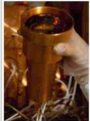
Second upgrade at end of 2010: all PMTs replaced with new ones of higher Q.E.
