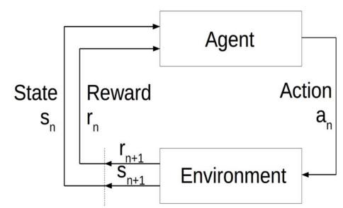
Reinforcement learning is a framework to find a good (optinal) POLICY for achieving given long-term tasks. It is widely used in artificial intelligence and machine learning. It is based on the interaction between a decision-maker (in our case the inertial particle) and the environment. The decision maker can change its behaviour in response to inputs from the system. By trial and error the decision maker progressively learns how to behave optimally
