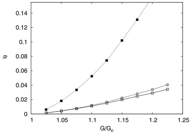
FIG. 8. Surface tension as a function of the interaction parameter  $\mathcal{G}_b$ . The surface tension calculated using both expressions in Eq. (43), the case with  $\partial_y \rho$  (○) and the case with  $\partial_y \psi$  (□). To show the importance of the normalization factor (42) we also show the surface tension calculated by simply replacing  $\partial_y \psi \rightarrow \partial_y \rho$  in (28) (filled squares).
