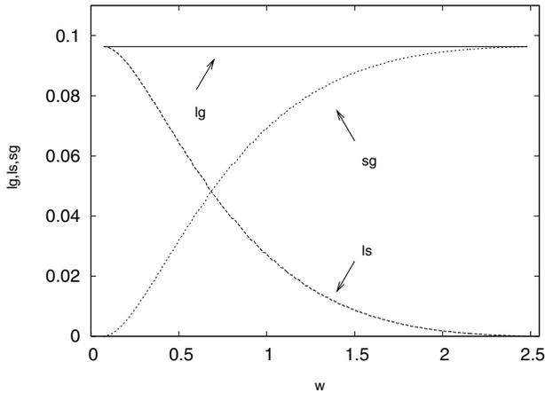
FIG. 2. Surface tensions in a three phase system for  $\mathcal{G}_b = -6.0$  as a function of  $\rho_w$ . The horizontal line represents the surface tension between liquid and gas ( $\gamma_{lg}$ ). The surface tension between solid and gas ( $\gamma_{sg}$ ) is zero for  $\rho_w = \rho_g = 0.07$  and equal to  $\gamma_{lg}$  for  $\rho_w = \rho_l = 2.65$ . The surface tension between liquid and solid ( $\gamma_{ls}$ ) reflects the opposite behavior.
