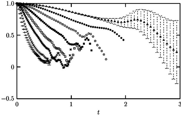
FIG. 4. Modulus of the average response functions,  $G_n^n(t) = \langle R_n^n(t) \rangle$ , for shells  $n=7, \dots, 14$  (from top to bottom). Error bars are shown only for the smallest and the largest scales. The number of independent kicks used to perform the averages is around  $2 \times 10^5$ . Notice the extremely large error bars measured for the slowest shell variables. The parameters entering in the equations of motion (14) are  $b=0.4$ ,  $\nu=5 \times 10^{-7}$  for  $N=25$  shells.
