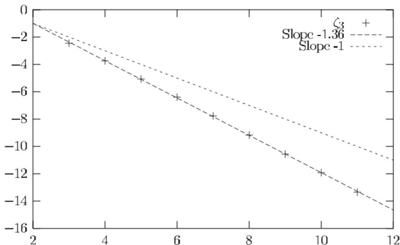
Fig. 2. Log-log plot of measured scaling of  $S_3(n)$  vs.  $n$  for a time dependent binomial random multiplicative process. The slope fitted slope  $\zeta_3 \simeq -1.36$  is “renormalized” with respect to the “bare” value  $\zeta_3 = 1$ .
