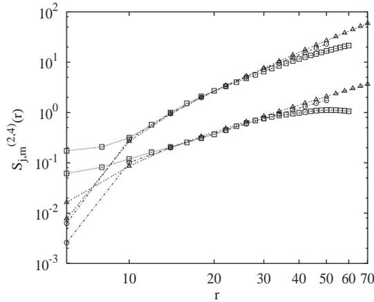
Fig. 1. Log–log plot of the most intense anisotropic sectors for structure functions of order 2 and 4, at different Reynolds numbers and different large-scale forcing. Top three curves:  $S_{2,2}^4(r)$  at  $Re_\lambda = 60$  ( $\circ$ ) and  $Re_\lambda = 90$  ( $\triangle$ ) for the RKF, and for flow 3 (see text) at  $Re_\lambda = 90$  ( $\square$ ). Bottom curves,  $S_{4,0}^2(r)$  for the same three cases.
