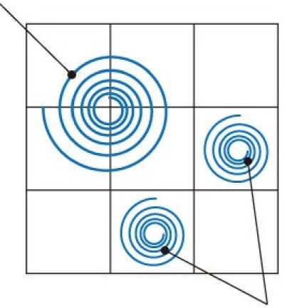
Sub-Grid Scale (SGS): Not captured by the grid Needs to be modeled
