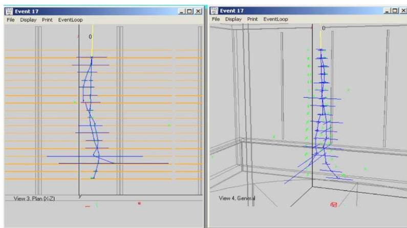
Fig. 3. 100 MeV gamma tracked in the GLAST-LAT.
