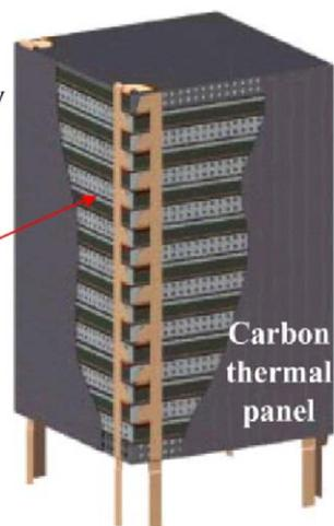
Fig. 2. The GLAST tracker tower.
