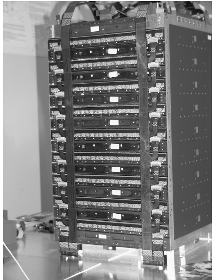
Fig. 1. A tracker tower during the assembly. The trays structure and the front–end electronic boards are visible.
