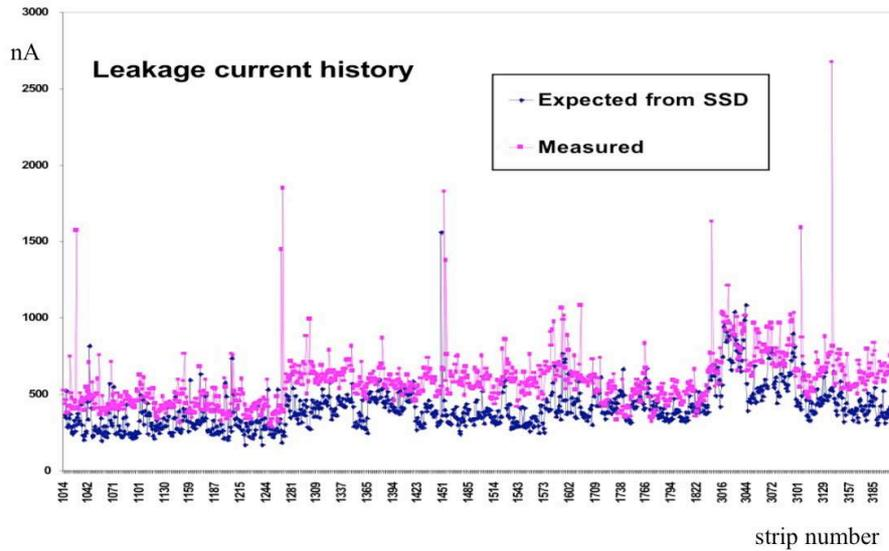
Figure 4: History of the expected and measured leakage currents of LAT Ladders. The values above 1000nA indicates a bad connection of the wafers within the ladder
