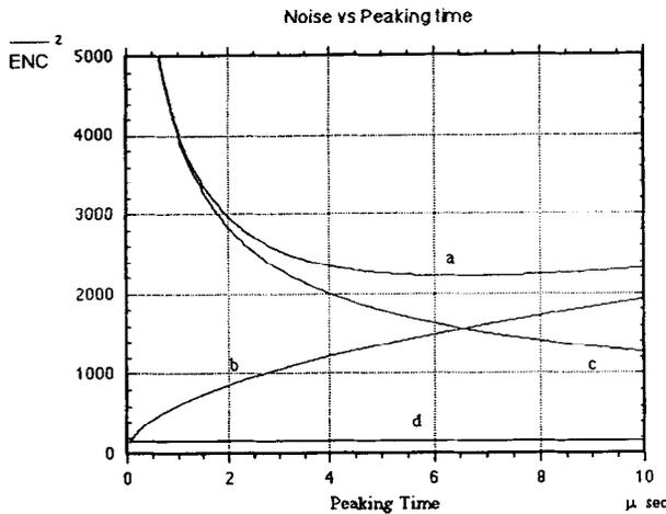
Fig. 7. Front-end electronics: Equivalent Noise Charge (ENC) vs. peaking time. The curves displayed are: a: total noise; b: current noise; c: shot noise; d:  $1/f$  noise. The chosen working point is  $7 \mu\text{s}$ .
