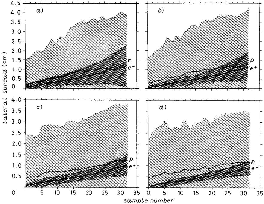
Fig. 2. — Estimated variance of the projected coordinate, as a function of the order number of the samples and for different energies,  $E_{inc}$ , of the incident particle. a)  $E_{inc} = 10$  GeV; b)  $E_{inc} = 20$  GeV; c)  $E_{inc} = 50$  GeV; d)  $E_{inc} = 100$  GeV. Solid lines represent the mean values for proton (p) and for positrons ( $e^+$ ). Dashed areas represent the regions where 95% of the events are contained.
