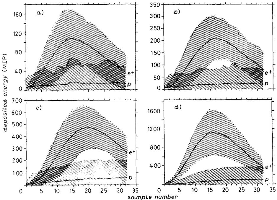
Fig. 1. – Deposited energy—in the sensitive layers of the calorimeter—as a function of the order number of the samples and for different energies,  $E_{inc}$ , of the incident particle. a)  $E_{inc} = 10$  GeV; b)  $E_{inc} = 20$  GeV; c)  $E_{inc} = 50$  GeV; d)  $E_{inc} = 100$  GeV. Solid lines represent the mean values for proton (p) and for positrons ( $e^+$ ). Dashed areas represent the regions where 95% of the events are contained.
