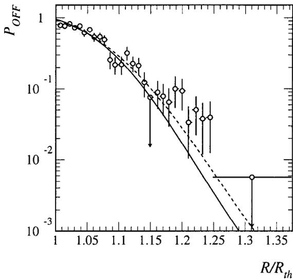
Figure 2. Probability  $P_{OFF}$  of detecting zero photoelectrons. Open circles: muons from ground data. Dashed curve: fit to experimental points. Solid curve: parameterization obtained after the correction for the spectrometer effect.
