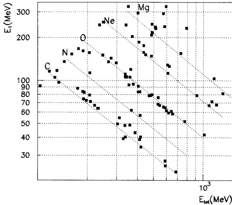
Fig. 4. Nuclear identification capabilities of the detectors NINA. Data refer to the 14 November 1998 SEP event, detected by NINA on board the satellite Resurs.
