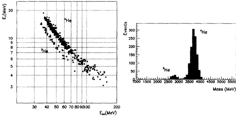
Fig. 3. NINA detector isotope identification capabilities.  ${}^3\text{He}/{}^4\text{He}$  data refer to 6-8 November 1998 SEP event, detected by NINA on board the satellite Resurs.
