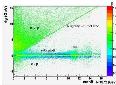
Figure 4: Rigidity vs Stormer Cutoff observed with PAMELA. Colour bar represents  $\beta$  of particles. The effect of the cutoff on galactic particles is clearly visible and well separated from reentrant albedo events, which have a rigidity below the expected cutoff.
