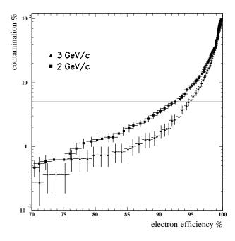
Fig. 4. PAMELA TRD hadron contamination versus electron detection efficiency from a beam test performed at CERN PS.
