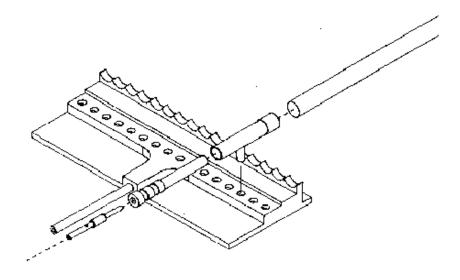
Fig. 3. Exploded view of a straw tube connection to the gas manifold plate and HV connector.
