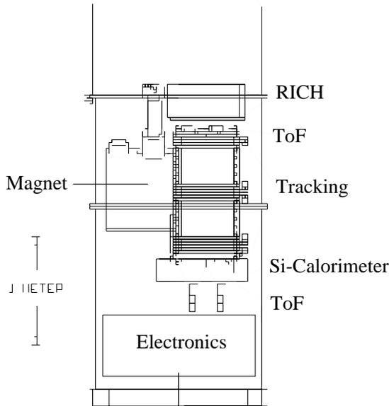
Figure 1. The CAPRICE apparatus in the 1994 configuration (CAPRICE94).
