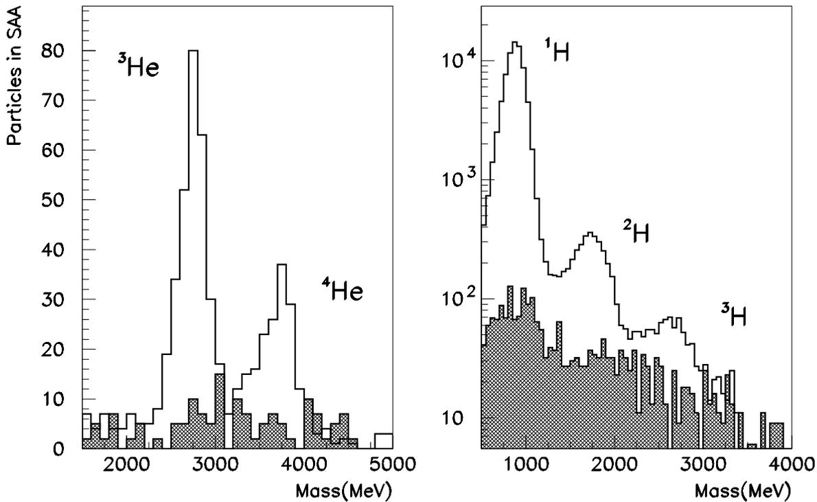
**Fig. 1.** Mass distributions for geomagnetically trapped He (left) and H (right) isotopes measured at L-shell < 1.2 and  $B < 0.22$  G. The shaded area represents the estimated background. Arbitrary units on Y axis.
