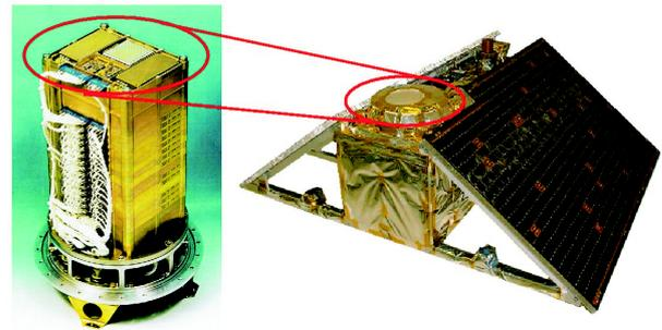
**Fig. 1.** The NINA-2 detector (left - height: 48 cm, diameter: 28 cm) and its accommodation within MITA satellite (right). MITA is three-axis stabilized with the detector pointing toward the zenith.
