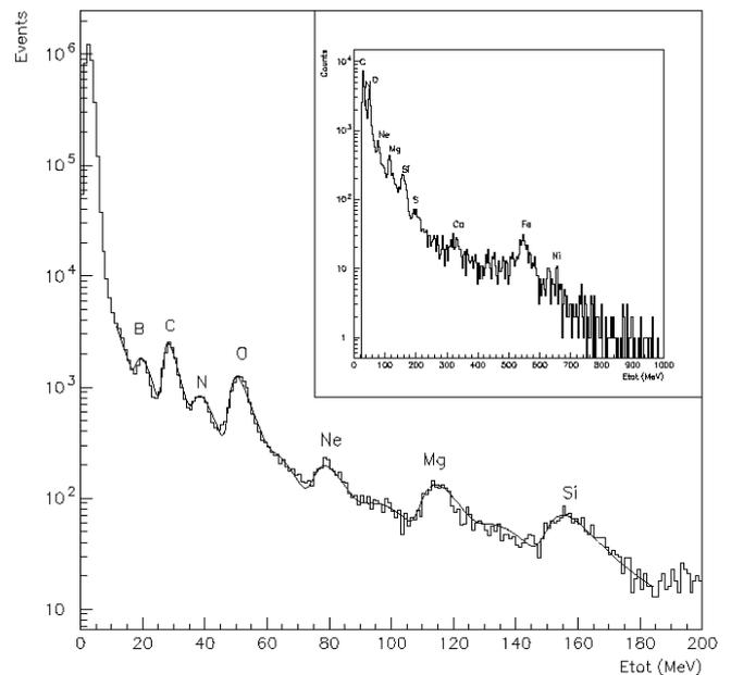
**Fig. 2.** Nuclear identification capabilities of SilEye-2 for nuclei up to Si. In the inset is shown the contribution of nuclei up to Ni. The continuous line corresponds to a fit using a Landau distribution per nuclear species (see text).
