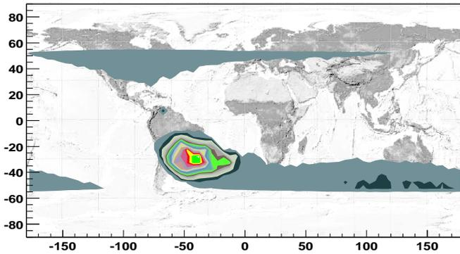
**Fig. 1.** Acquisition rate as a function of position (Y: latitude - degrees, X: longitude - degrees) for all solar quiet sessions. It is possible to see the increase in the SAA region. Each contour level represents a flux increase of 3 Hz.
