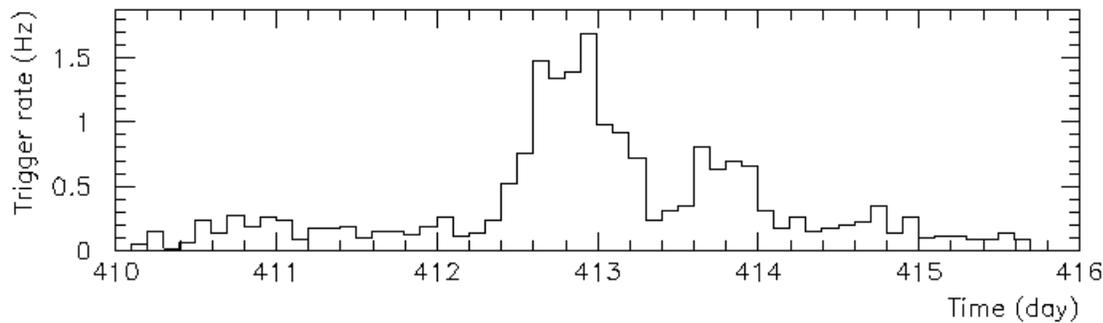
**Figure 4:** Detection of a solar flare by NINA. Data are restricted to particles detected in polar regions. It is possible to see the flux increase associated to the arrival of the flare at 1AU on day 412.4 (February 16) and the subsequent return to quiet time values in the following days.
