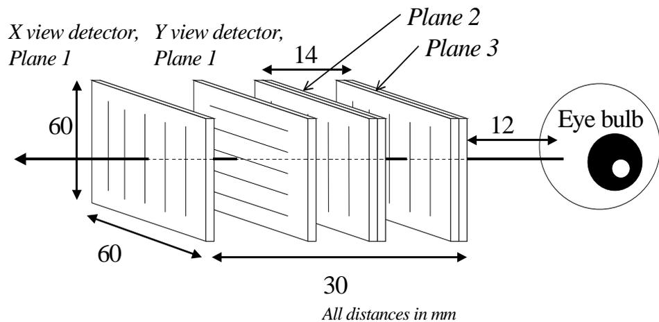
**Figure 1.** Silicon detector setup scheme for SilEye-2 (see text for details). Passive Iron absorbers of 1 mm interposed between planes are not shown.
