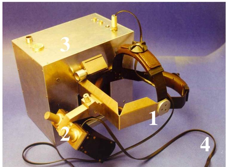
**Figure 2:** The SilEye2 apparatus: 1. Head Mounting 2. Eye mask 3. Detector box (it is placed on one side of the head). 4. Connection cables for dark adaptation LED.
