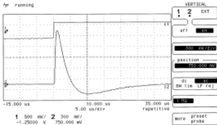
**Figure 4:** Scope picture showing the analog output of one channel of a CR1.3 chip (trace 2) corresponding to an input calibration signal (trace 1) equivalent to about 300 MIPs.
