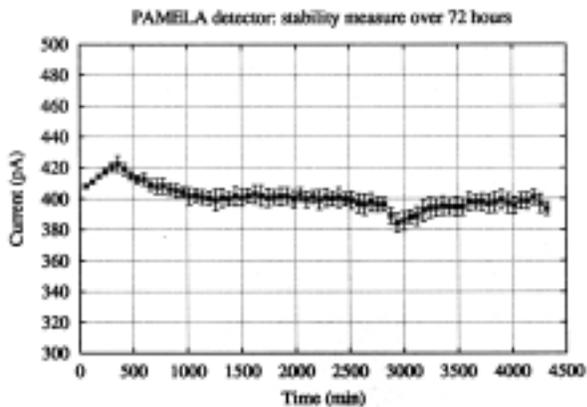
**Figure 3:** Stability measurement (at a depletion Voltage of 90 V) of the leakage current for a PAMELA detector over 72 hours.
