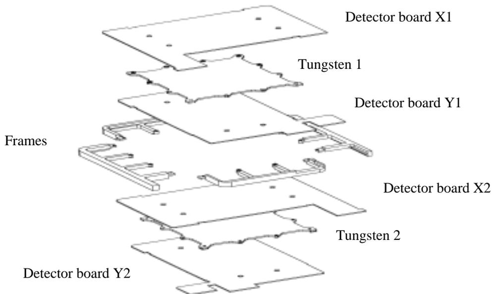
**Figure 1:** Exploded view of one detection module, showing the tungsten plates, the detector printed circuit boards and the supporting frames.
