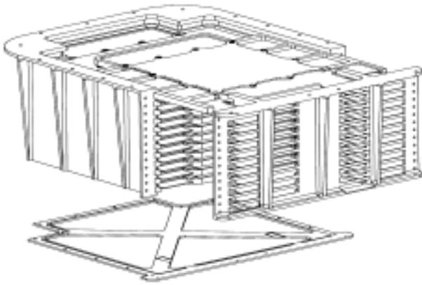
**Figure 2:** An assembly view of the mechanical structure of the calorimeter, showing also the locking front cover.
