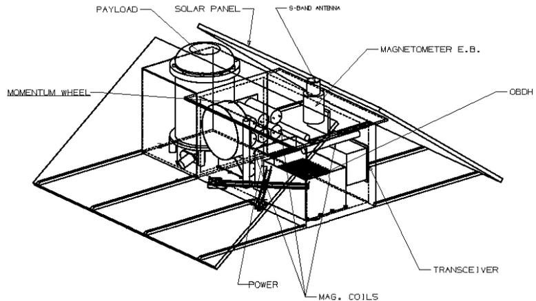
**Figure 1:** MITA internal layout – The configuration of the satellite is based on a cubic shaped module and is designed especially for Low Earth Orbit missions.
