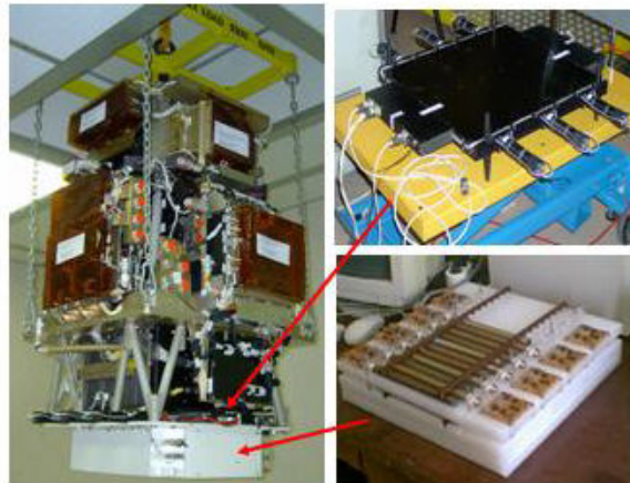
Figure 1. Left: view of the PAMELA flight Model. Right: [top] view of the bottom scintillator S4, [bottom] view of the neutron detector.
