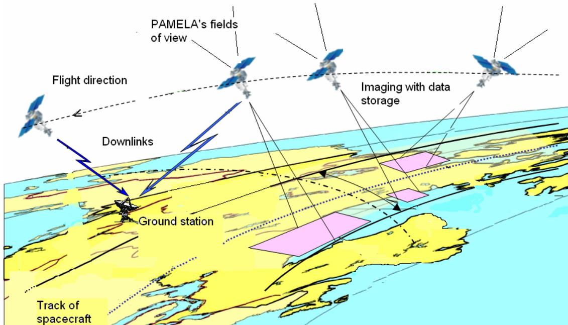
**Figure 1.** Data taking and downlinking during flight.
