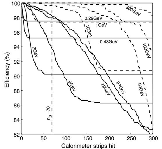
Fig. 9. The efficiency  $\eta$  of the L2 trigger is shown as function of  $n_s$  for simulated protons (solid lines) and electrons (dashed lines) of several energies. The efficiencies for the chosen value  $n_s = 70$  (dash-dot line) correspond to the values shown in Fig. 10 (bold line).
