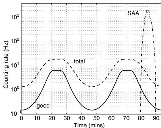
Fig. 6. The PAMELA trigger rate evaluated during an arbitrary orbit (period  $\sim 94$  min). The dotted curve is an estimation of the total trigger rate, while the lower curve shows only the good triggers. The trigger rate is strongly dependent on the orbital position, and reaches a minimum in equatorial regions. The sharp increase in the trigger rate towards the right of the plot is due to the South Atlantic Anomaly (SAA). Adapted from [15].
