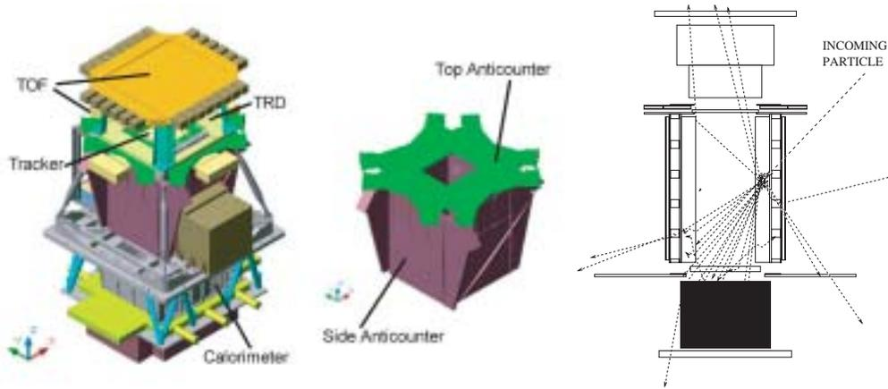
**Fig. 1.** Left: a stylised view of the PAMELA experiment showing the location of the anticounter system. PAMELA is approximately 1.2 m tall. Right: a simulation of a false trigger. A proton enters PAMELA from the side and interacts in the magnet producing secondaries which give coincidental energy deposits in the time-of-flight scintillators thereby producing a trigger.
