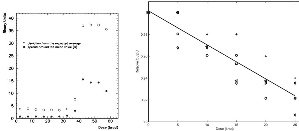
**Fig. 3.** Left: The effect of ionising radiation on the expected ADC output. At a dose 6 times higher than expected during the PAMELA mission (30 krad) the ADC chip malfunctions. Right: The output intensity of a selection of LEDs tested for the anticounter calibration system. An attenuation of approximately 10 % is seen after 30 krad.
