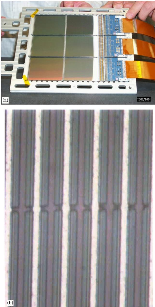
Fig. 2. (a) Complete tracking plane. (b) Example of implantation defects found on the P-side of the first set of microstrip silicon sensors of the tracking system.
