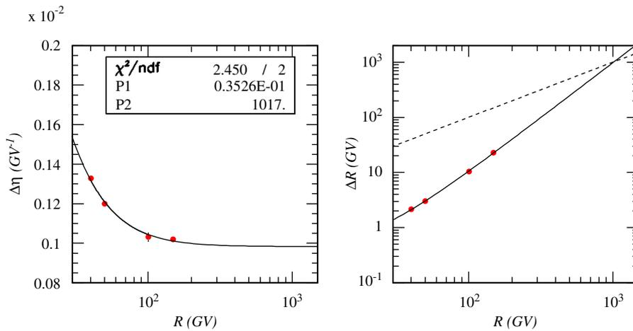
Fig. 4. Results of a test at SPS (CERN) using a proton beam. Uncertainties on the deflection  $\eta$  (left) and on the rigidity  $R$  (right) as functions of  $R$ .
