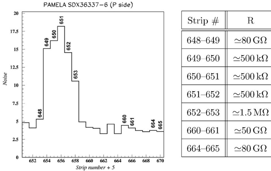
Fig. 3. Left: electronic noise (in ADC channels) for a group of microstrips around the bad ones; strip numbers are indicated over the histogram bars. Right: table of interstrip resistance values for the same group of microstrips.
