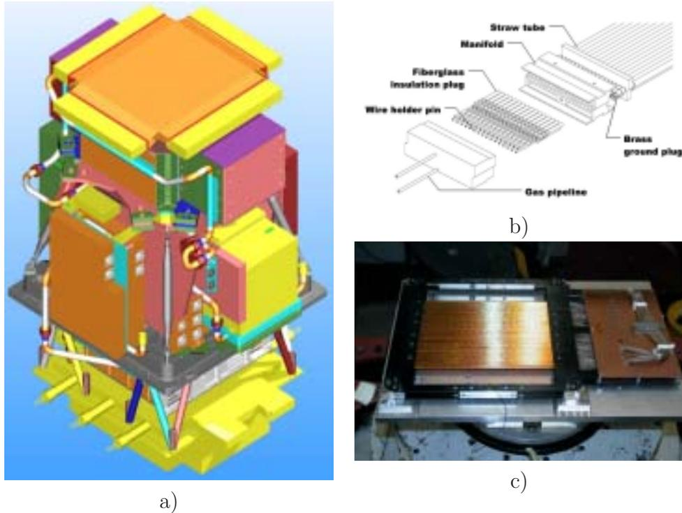
**Fig. 1.** a) A 3D view of the PAMELA instrument. b) Detail of a module assembly. c) A sensitive plane, without radiator.
