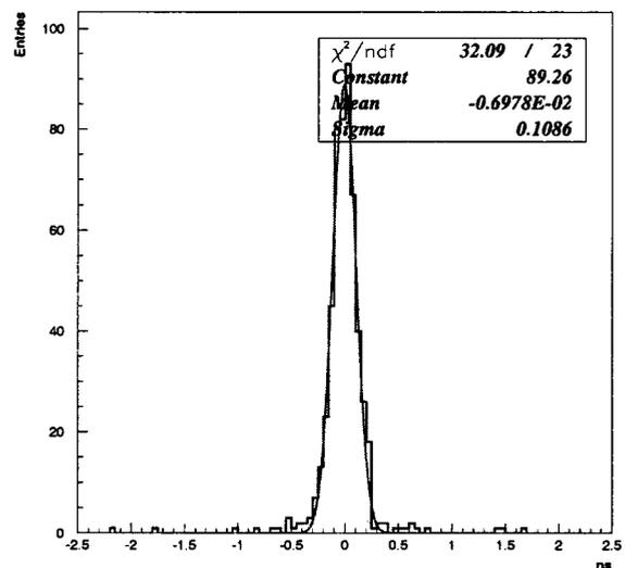
Figure 3. Result of time resolution measurements on a counter of the S1 layer.
