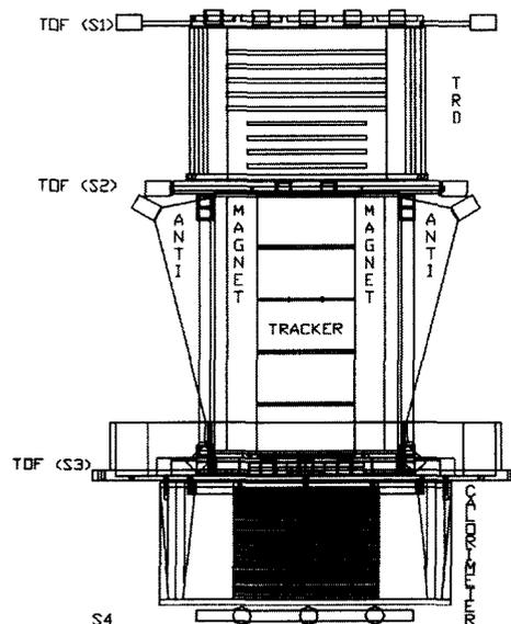
Figure 1. The **PAMELA** apparatus (1050 mm high) consists of a transition radiation detector (TRD), a magnetic spectrometer equipped with silicon micro-strip detector, a silicon/tungsten calorimeter, a time-of-flight detector (TOF), and an anti-coincidence system (ANTI).
