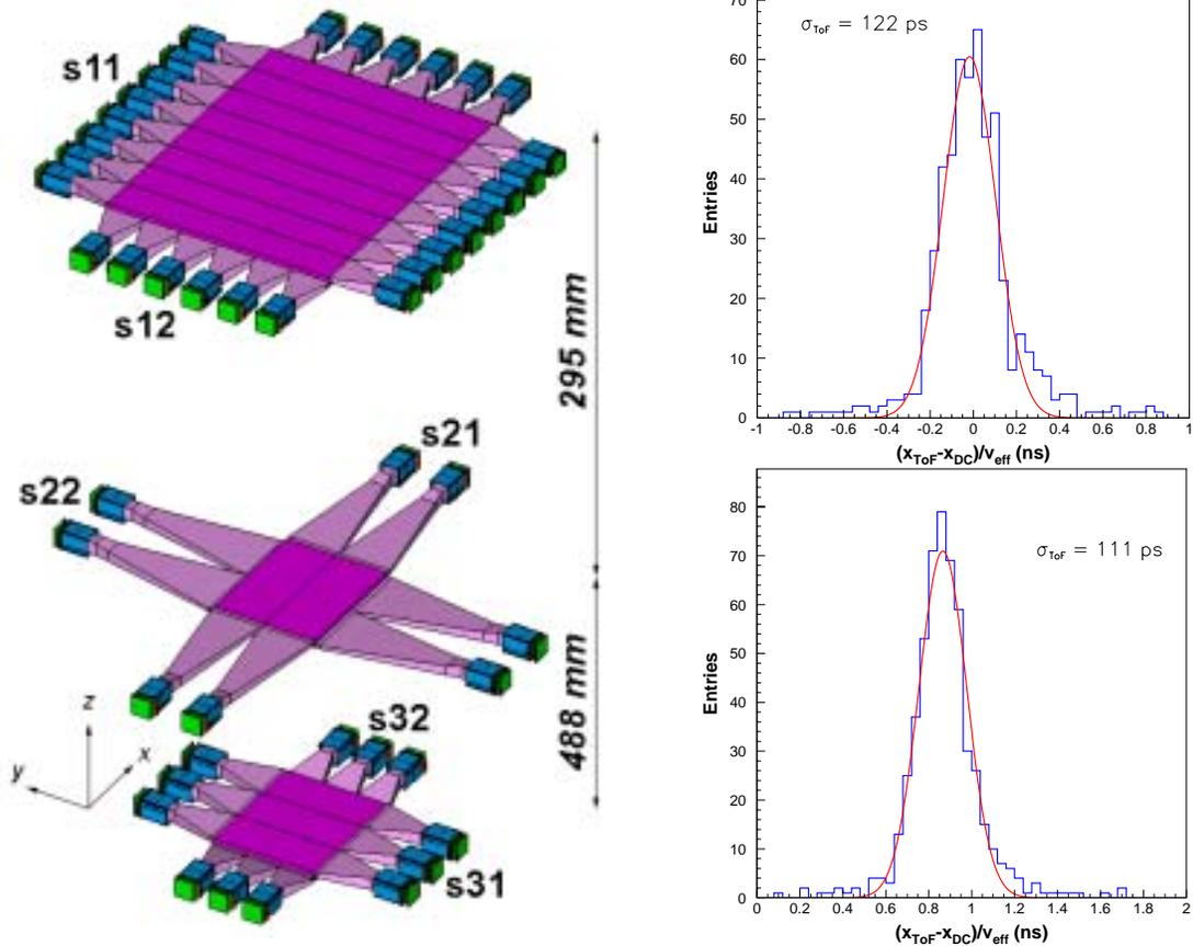
**Fig. 1.** Left: isometric view of the ToF. Right: sample time resolution of a ToF paddle before (above) and after (below) time-walk correction.
