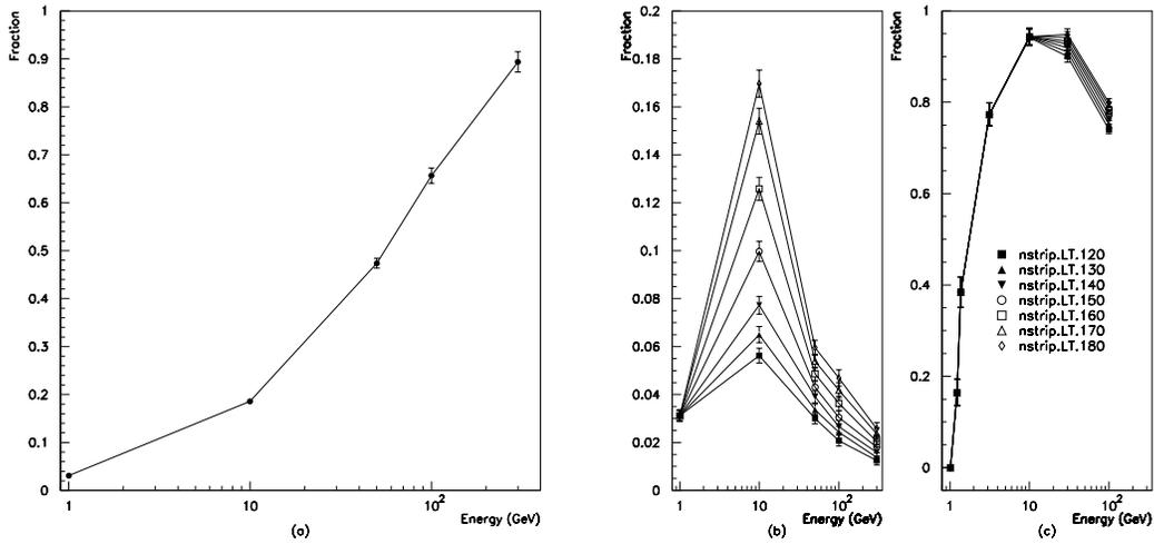
**Fig. 2.** a) Backscattering ratio with only AC rejection (electrons), b) Backscattering ratio with combined AC and calorimeter rejection (electrons), c) Rejection ratio with combined AC and calorimeter rejection (protons)
