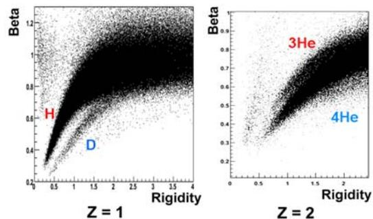
Fig 6: Mass separation for  $Z=1$  and  $Z=2$  particles with the  $\beta$  vs. rigidity method.
