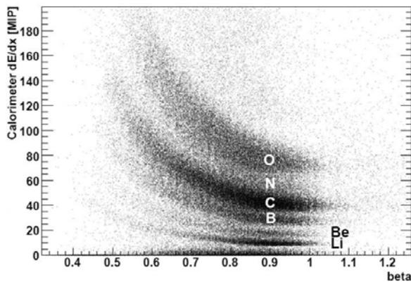
Fig 4: The ionization loss in the first plane of the calorimeter vs. the particle velocity.
