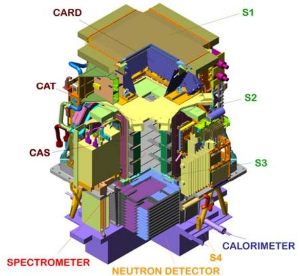
Fig 1. Schematic overview of the PAMELA apparatus. The detector is approximately 1.3 m high, has a mass of 470 kg and an average power consumption of 355 W.
