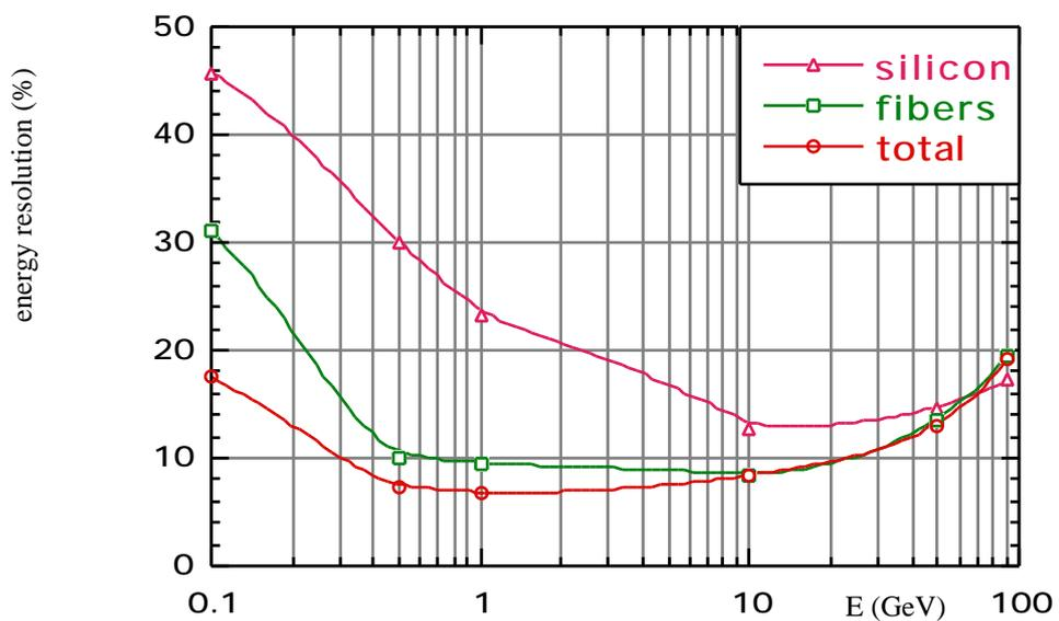
Figure 7. Simulated behaviour of GILDA energy resolution as a function of energy for lead fibers (squares), silicon strips (triangles) and total (sum of the two: bullets).
