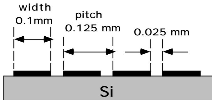
Figure 2. *The 125 micron silicon strips.*
