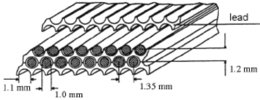
Figure 4. Structure of the lead scintillating fibers.
