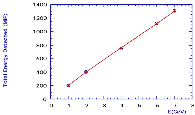
Figure 5. Energy linearity of the prototype of the WiZard calorimeter; real data (triangles), MC data (bullets).
