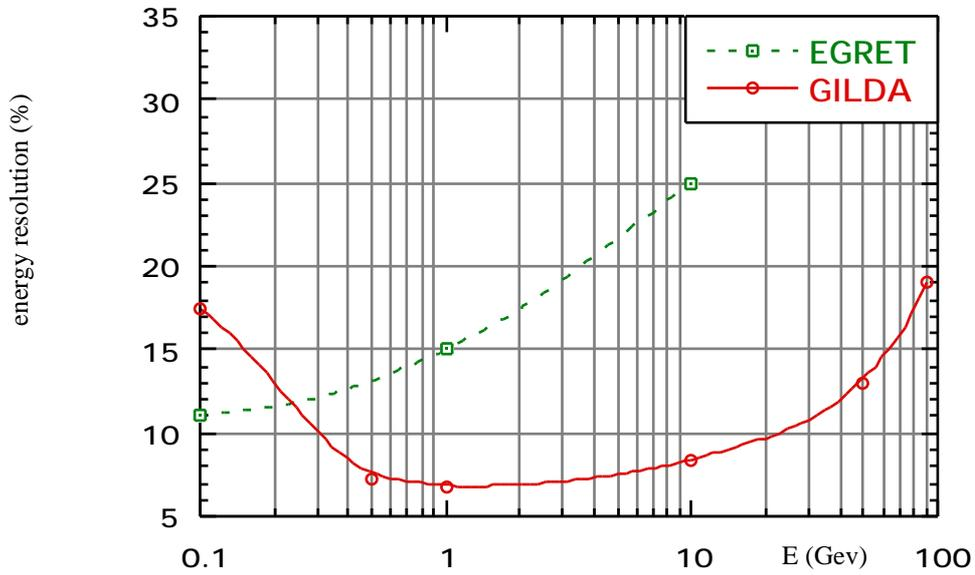
Figure 8. Simulated GILDA energy resolution, compared with EGRET.
