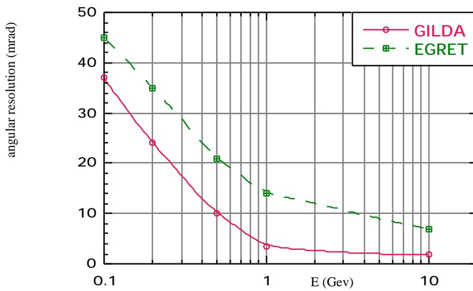
Figure 10. *Simulated GILDA angular resolution, compared with EGRET.*
