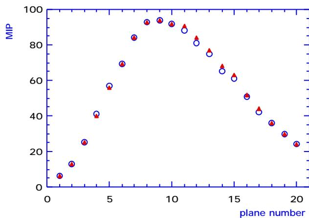
Figure 6. Longitudinal development of an electromagnetic shower for the prototype of the WiZard calorimeter; real data (triangles), MC data (bullets).
