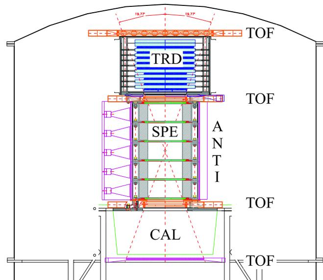
Figure 1: *the PAMELA telescope. The main detectors are: a transition radiation detector (TRD), a permanent magnet spectrometer equipped with silicon micro-strip detector (SPE) and a silicon/tungsten calorimeter (CAL). There are also a time of flight detector (TOF) and an anti-coincidence system (ANTI) made by plastic scintillator.*
