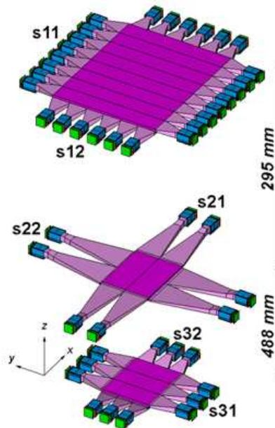
Figure 2: Isometric view of the ToF planes.
