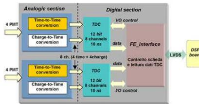
Figure 6: Block diagram of a FE board.
