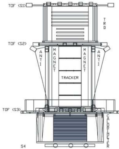
Figure 1: Schematic drawing of the PAMELA apparatus.
