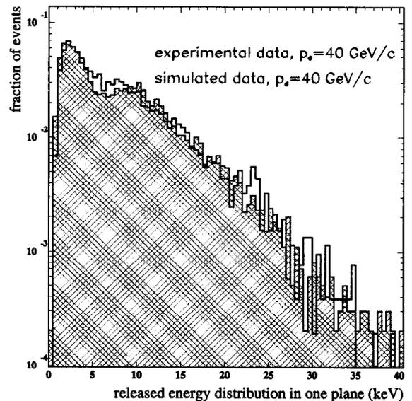
Figure 4. Distribution of the energy detected in a plane of the TRD from 40 GeV/c pions (upper plot). Distribution of the energy detected in a plane of the TRD for 40 GeV/c electrons (lower plot). The contribution of the transition radiation is clearly visible in addition to ionization above about 4 keV.
