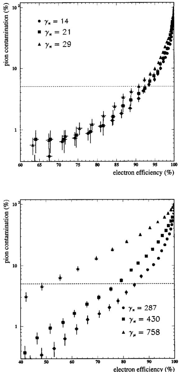
Figure 5. Pion contamination versus electron efficiency for the PS data (upper plot). Pion and muon contamination versus electron efficiency for the SPS data (lower plot).
